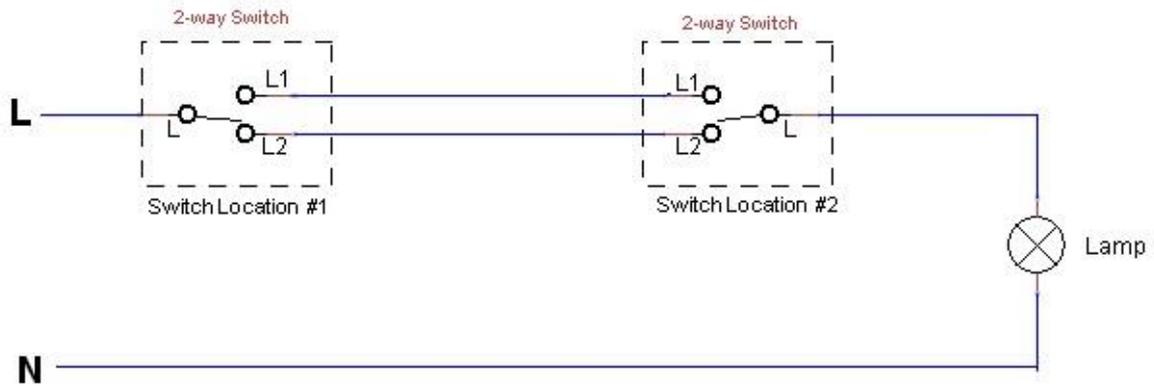
**Note:** "LOOP" terminal if present - no connection, unless the Neutral loop wire is at switch location
